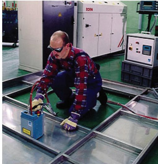
Welding of large sized thin metal sheets
