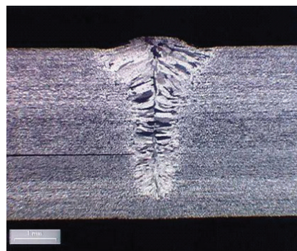
Metallographic samples of typical laser beam welded seams left: overlapped weld, right: square butt weld
